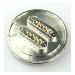
Please note: The 5-pin power and coaxial feedthroughs are not symmetrical, BUT you can turn an air side connector by 180° to fit on the vacuum side. The housings are made to accept this. Please mind, that the pin numbering shown on the connectors is no longer valid in this case.
