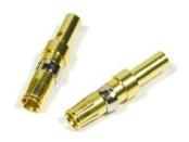
High Voltage pins can be used for in-vacuum connections either on its own or with Mixed male and female connectors. The in-vacuum voltage rating is 5KV DC. Test voltage 10KV in vacuum. Air side use max. 2,7KV DC
